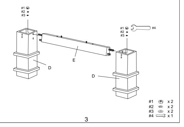
Step 3. Attach table supports (part F) to pedestals (part D) using large flat washers (part #3), large spring washers (part #2), hex nuts (part #1) and wrench (part #4).
